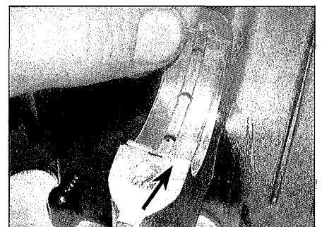
25.11 Press each shell into place, locating the tab in the notch (arrowed)
