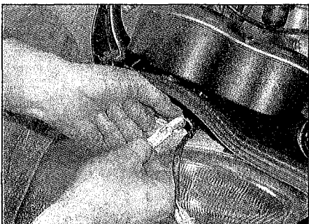
3.18c . . . and disconnect the LED if fitted
