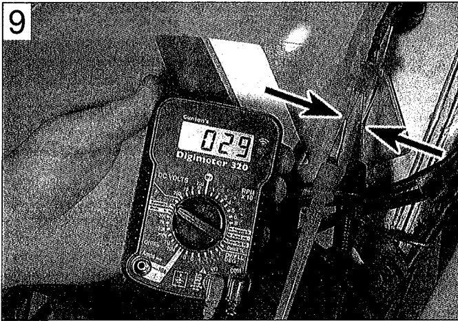
9 Continuity check of front brake light switch using a meter - note split pins used to access connector terminals
