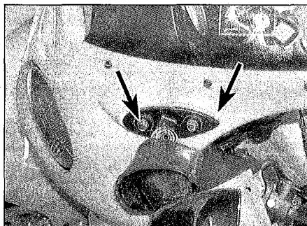
4.3c Mirror mounting bolts (arrowed)
