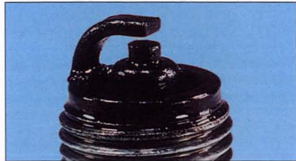
Oil fouling – Wet oily deposits leading to misfire and weak spark. Caused by oil leakage past piston rings or valve guides (4-stroke engine), or excess lubricant (2-stroke engine).
