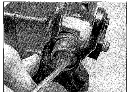
5.11c Remove the rubber boot from the end of the master cylinder piston . . .
