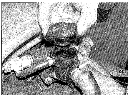
6.7 Remove the pressure cap from the filler neck as described
