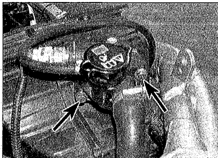
5.8 Thermostat cover bolts (arrowed) – Daytona shown
