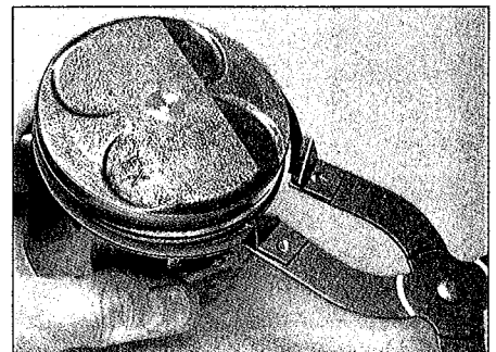
15.6 Removing the piston rings using a ring removal and installation tool
