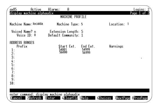
Figure 12-3. Machine Profile Screen for the Local Machine
