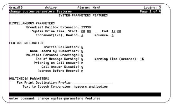
Figure 10-3. System-Parameters Features screen, Page 2; Setting Text-to-Speech Choices
