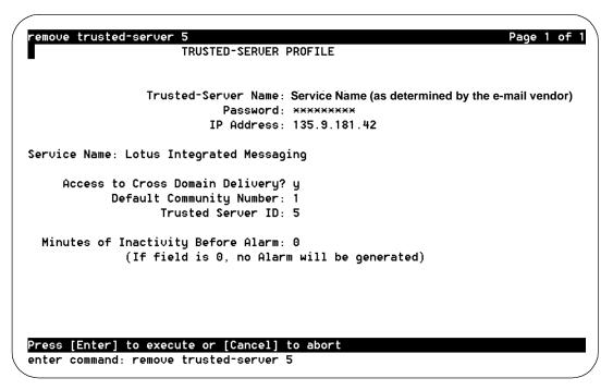
Figure 10-4. Trusted-Server Profile Screen; Defining a Trusted Server to the Lucent **INTUITY System**
