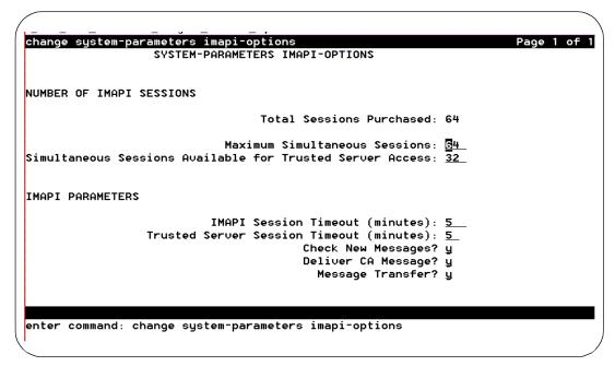
Figure 10-1. System-Parameters IMAPI-Options screen, Page 1; Setting IMAPI Sessions for Trusted Server Access
