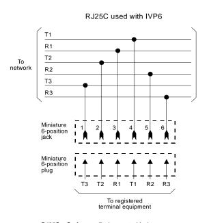
RJ25C - Surface- or flush-mounted jack
