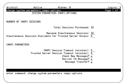
Figure 8-10. Change System-Parameters IMAPI Options Screen
