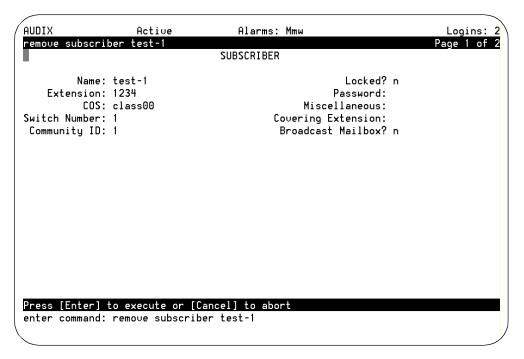
Figure 7-8. Remove Test Subscriber Screen
