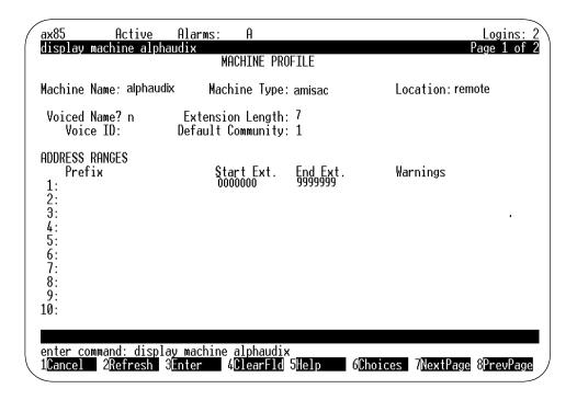
Figure 12-11. Machine Profile Screen for a Remote AMIS Machine
