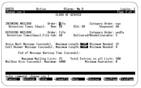
Figure 10-8. Subscriber Class of Service Parameters Screen, Page 2; Enabling E-mail on a COS Basis
