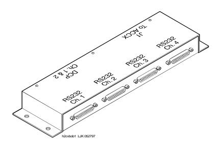
Figure 3-6. RS-232 Connections on a Breakout Box
