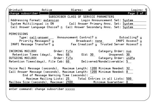
Figure 7-6. Subscriber Class of Service Parameters Screen
