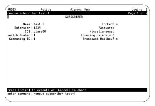
Figure 9-6. Remove Test Subscriber Window
