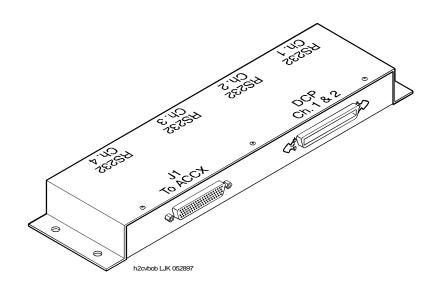
Figure 3-7. DCP Connections on a Breakout Box
