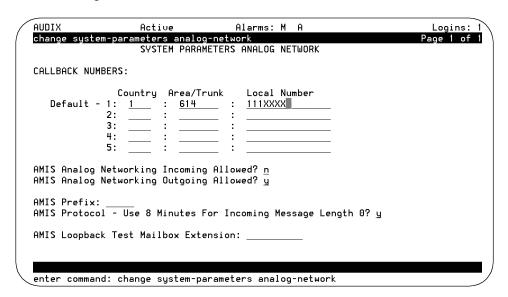
Figure 9-3. System Parameters Analog Network Screen
