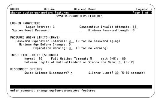
Figure 7-1. Change System - Parameters Features Screen, Page 1
