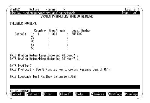
Figure 12-4. System-Parameters Analog-Network Screen
