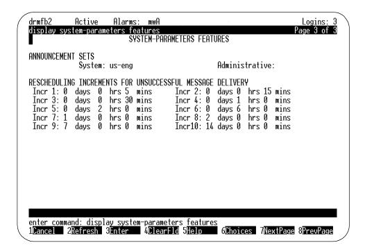
Figure 12-8. System-Parameters Features Screen (INTUITY AUDIX 3.2) — Page 3
