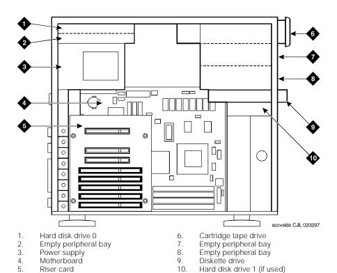
Figure 2-7. Side View of MAP/5P Including Locations of Peripheral Drive Devices
