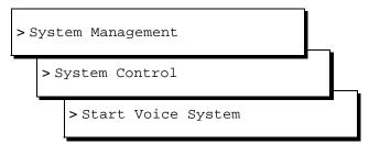
The system responds with a series of auditing messages. After the voice system is up, the system displays the following message: Press Enter to continue....Press (ENTER) to return to the system screens when you see this message.
