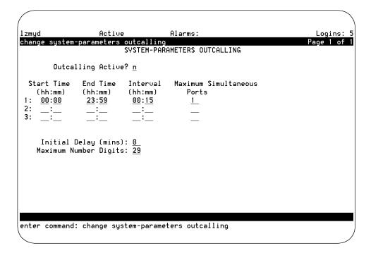
Figure 12-5. System-Parameters Outcalling Screen
