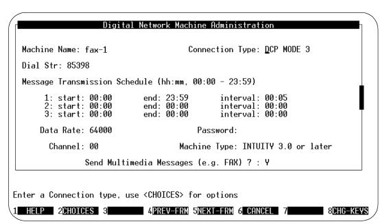
Figure 10-5. Digital Network Machine Administration Screen; Enabling a Remote Networked Machine to Receive E-Mail
