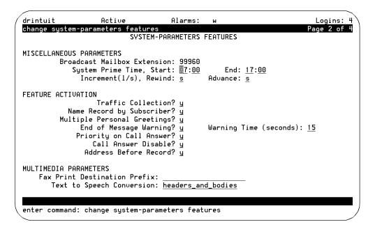
Figure 7-2. Change System-Parameters Features Screen, Page 2
