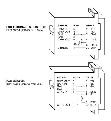
Figure D-3. Pinout Connections for DTE or DCE Devices
